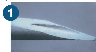
Syringe Needle AFTER TWO Uses
