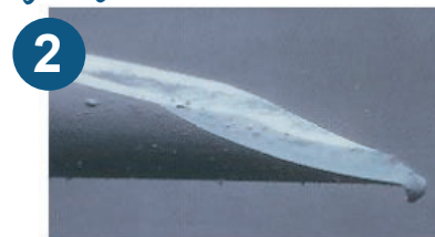
Syringe Needle AFTER TWO Uses
